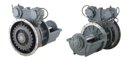
At the heart of the HP610S is an oil-filled, multiple disc, hydraulically-actuated self-adjusting clutch. Twin Disc's patented actuating technology facilitates seamless engagements and provides extraordinary durability resulting in long life and low maintenance.
